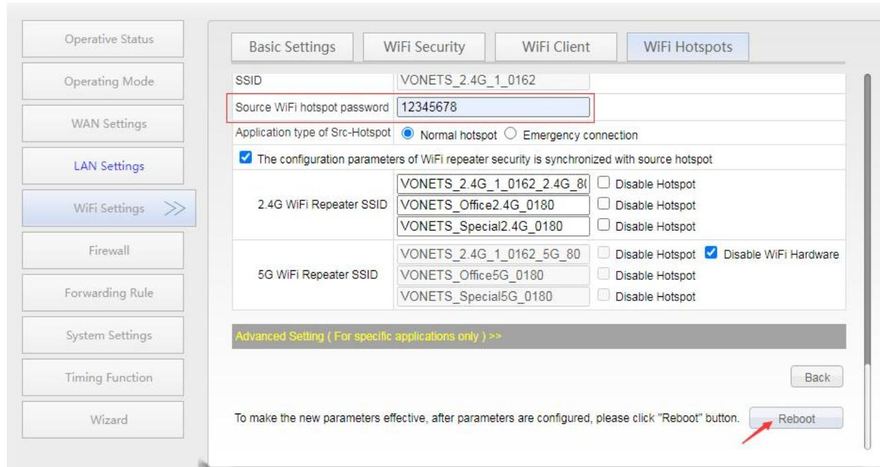
**Remark 3:** After VONETS device sets the WAN port to access the WiFi hotspot in the routing mode, its LAN port IP is still 192.168.254.254, and the terminal device also obtains the IP address of the same network segment, can login configuration page by 192.168.254.254 or <http://vonets.cfg>.
