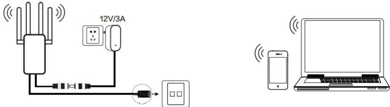
**1.2 Router Mode**(In the actual application environment, if the POE output port (PSE) is connected to a non-POE network port (PD is an access network port), please use it with caution, and ensure that the access network port is isolated from the power supply ground, otherwise it may cause the access device. damage!)
